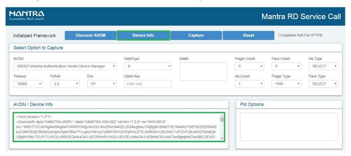
> By calling capture function of RD service, user can capture biometric data.
