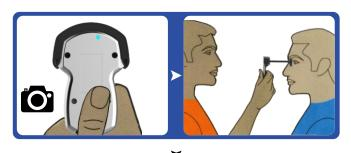
The rear light indicates the Camera is ON. Place the Guide Distance on the eye.
